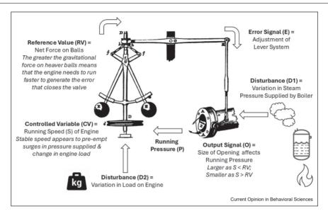
A diagram of a Watt's Governor that maps its components onto a PCT closed-loop model and explains how it appears to 'predict' how to respond to variations in load and pressure supplied without any capacity for prediction [15].
